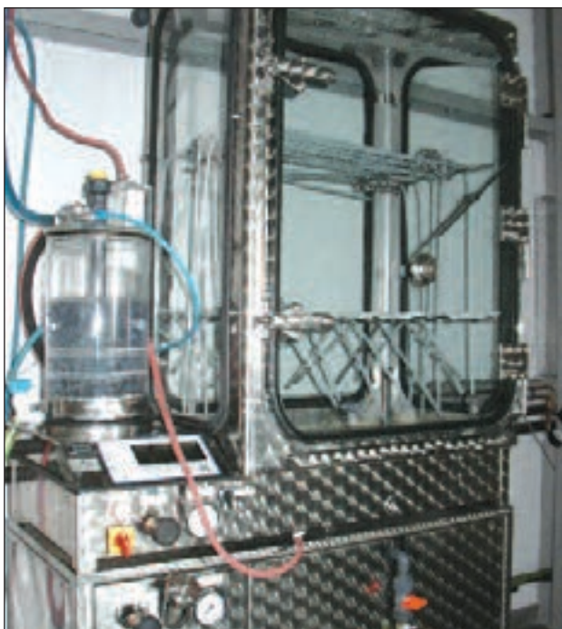
Figure 8.2: Environmental ageing chamber for ammonia atmosphere ageing
