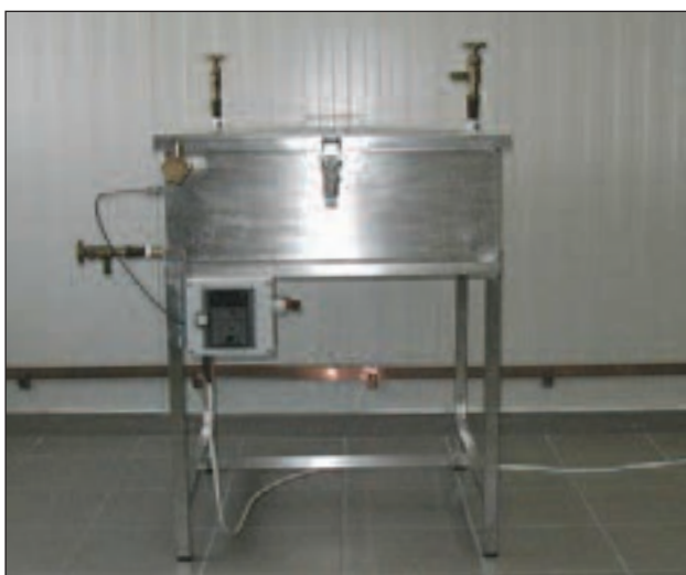
Figure 8.1: Environmental ageing chamber for salt mist and humid sulphurous atmosphere ageing
